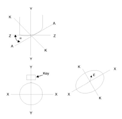
FIGURE 4. Ferrule end face geometry after polishing.
